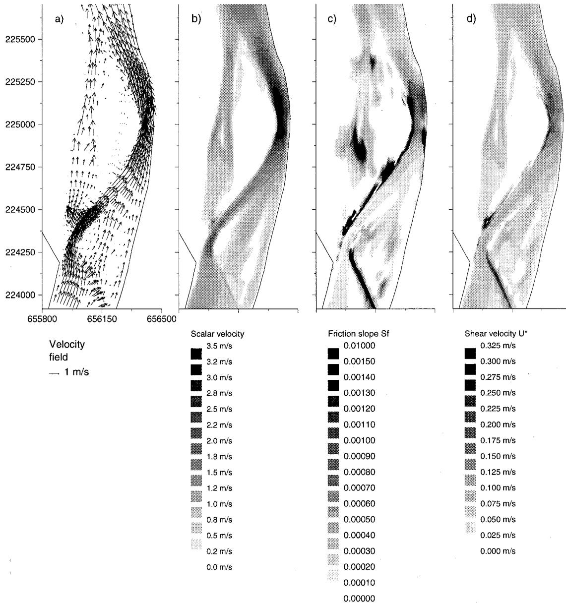
Figure 6. Indicators for morphological stability assessment. (a) Flow velocity field; (b) scalar value of velocity  $V$ ; (c) scalar value of the friction slope  $S_f$ ; (d) shear velocity  $U^*$
