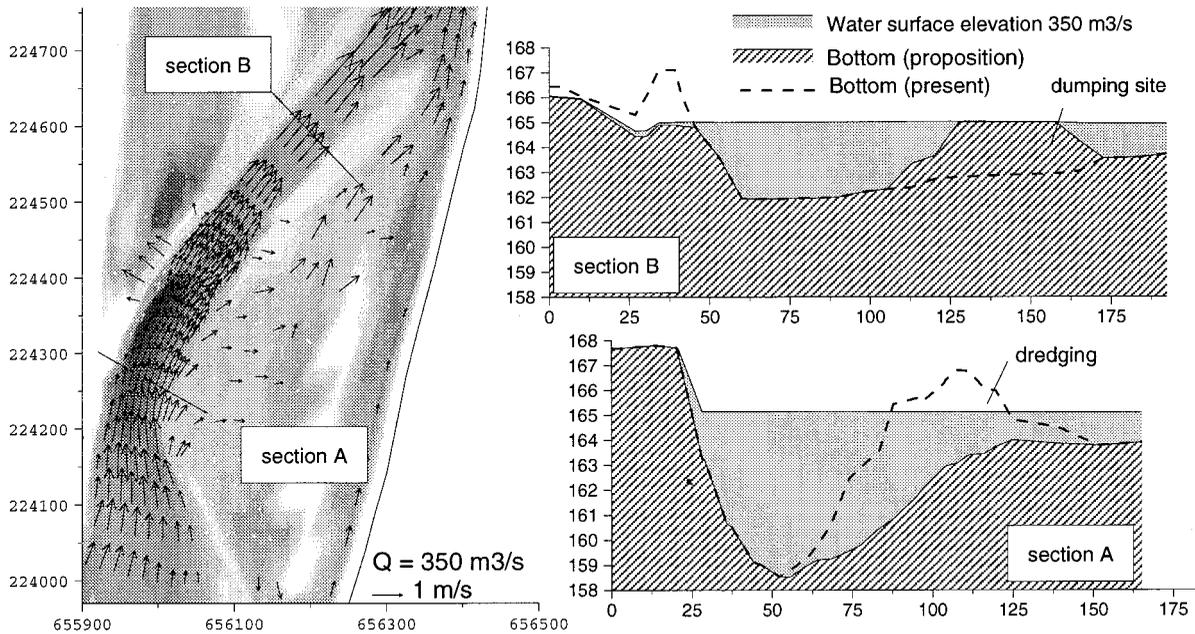
Figure 4. 'Chevette de Fourchambault': (a) Flow pattern; (b) cross section A, rectification and dredging upstream; (c) cross section B, dumping of dredged material
