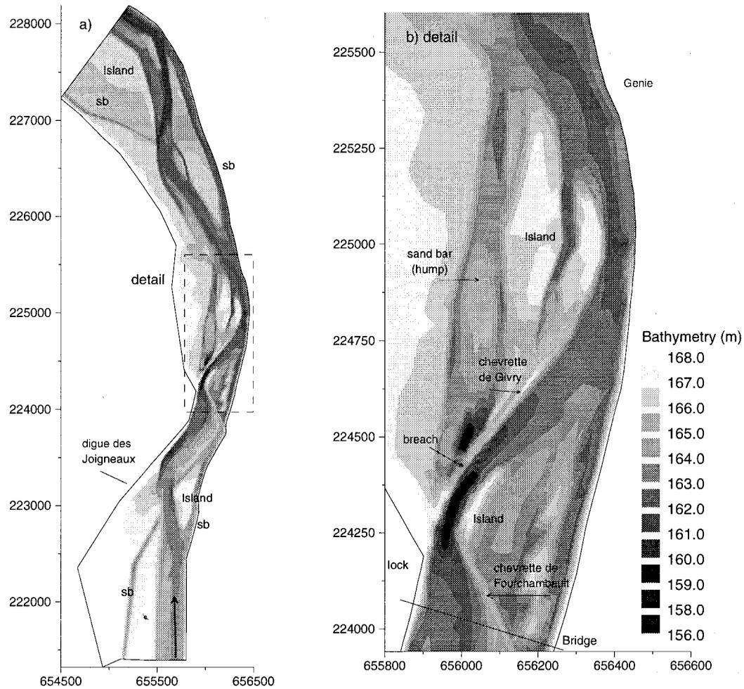
Figure 1. Site description and topography (plan views are referred to Lambert III Projection System in metres). (a) Full site, (b) detail of the central area
