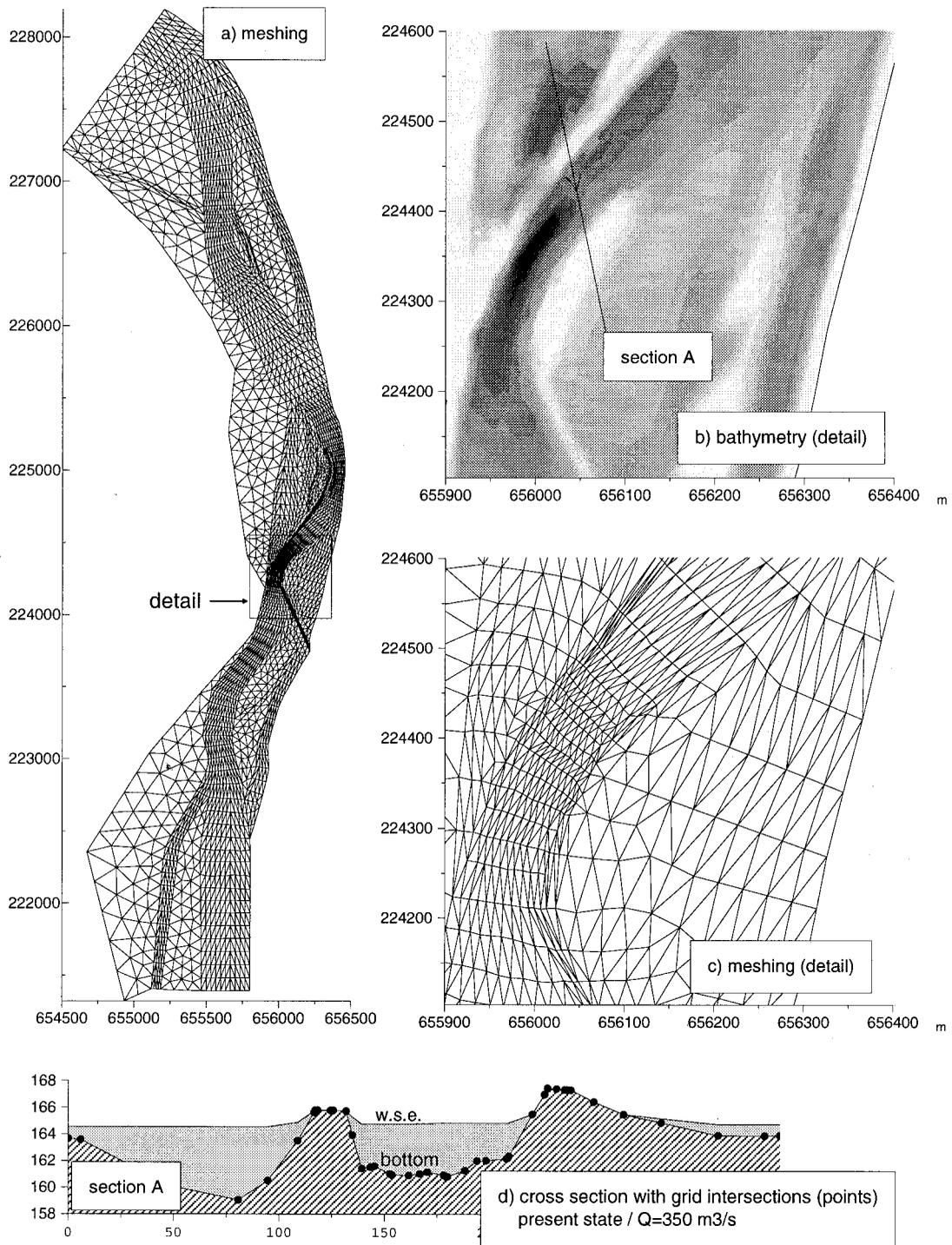
Figure 5. The computational grid of the model
