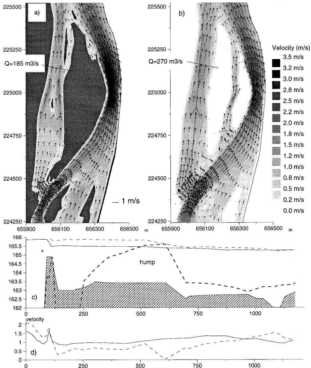
Figure 2. 'Chevette de Givry' total discharge =  $884 \text{ m}^3 \text{ s}^{-1}$ . (a) Present flow pattern; (b) after proposed modifications; (c) bottom and flow profiles (dotted lines: present; solid lines: proposed); (d) velocity profiles
