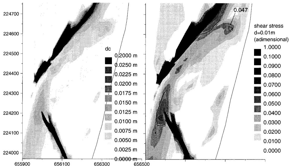
Figure 7. Indicators for morphological stability assessment. (a) Dimensionless shear stress; (b) critical sediment size
