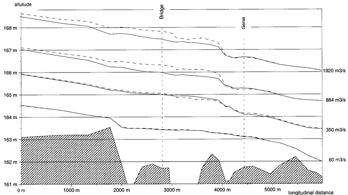
Figure 3. Flow lines along main channel (dotted lines: present—solid lines: proposed)
