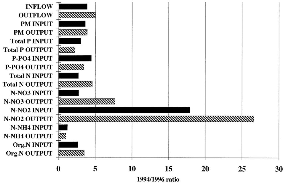
Figure 6. Annual differences of input and output of flow, PM, phosphorus and nitrogen (ratio of fluxes 1994/1996).
