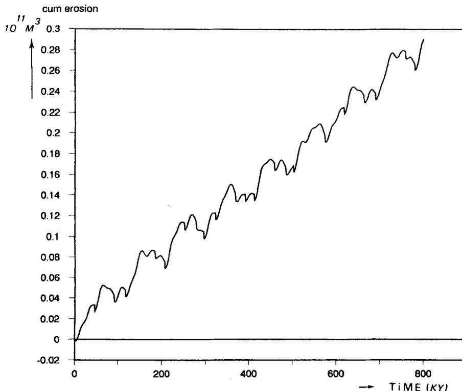
Figure 4. Cumulative erosion curve, derived from changes in discharge/sediment load equilibrium during simulation of LIMTER. This curve illustrates the alternating erosion and sedimentation stages during simulations
