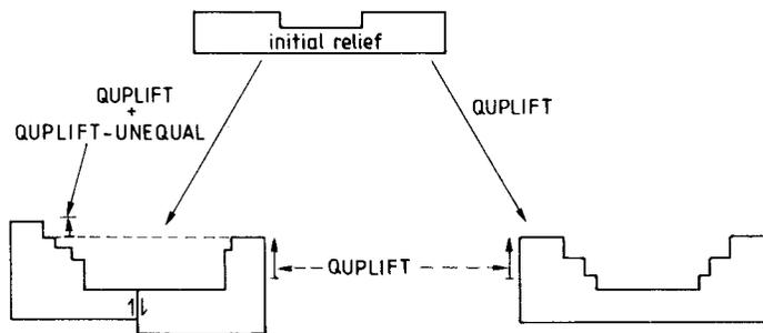
Figure 5. Two tectonic components as input of the LIMTER simulation. QUPLIFT is the general uplift of the modelled area, QUPLIFT-UNEQUAL is the difference in uplift rate between the two valley sides, assuming an active fault in the middle of the valley parallel to the flow direction
