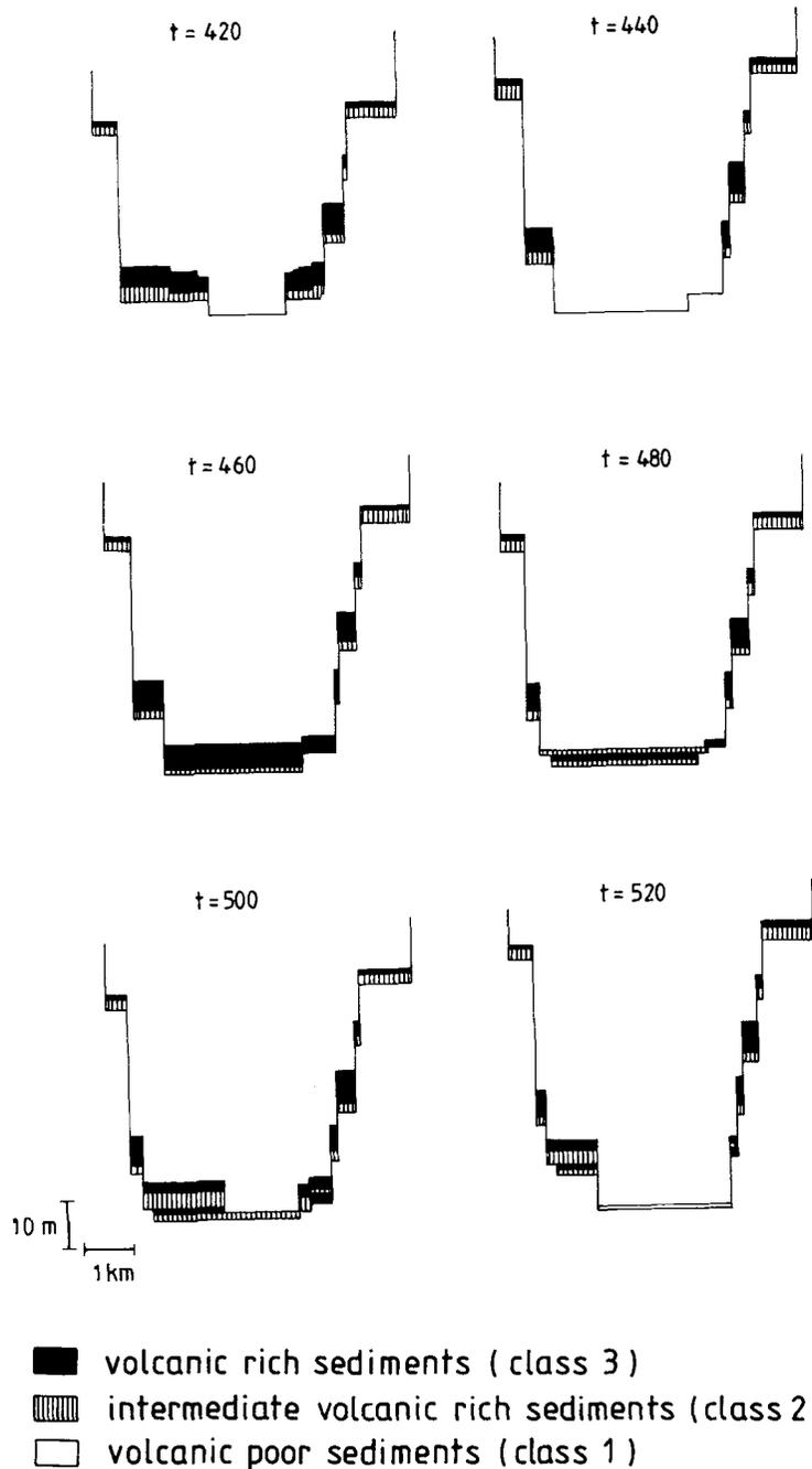
Figure 8. Cross section and terrace stratigraphy development during the last 100 ky of the simulation shown each 20 ky
