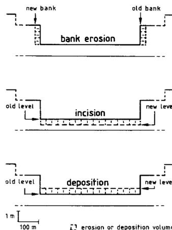
Figure 3. Cross section showing the impact of the model processes: incision, bank erosion and deposition
